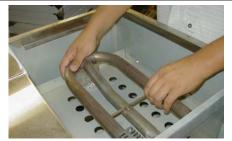
2-5) Replace the orifices #55, used for LP, and replace it with orifice #45, used for NG. Use a 1/2" Deep Socket and a Socket Wrench to remove and replace the orifice. Replace Griddle Plate Assembly when finished and re-install the Thermostat Bulb.
