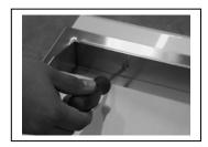
2-3) Raise the front of Griddle Plate Assembly and make sure the rear portion is resting on the Griddle Top as shown in the left picture. Pull out the Thermostat Bulb so that you may remove the Griddle Plate Assembly completely, as shown in the right picture.
