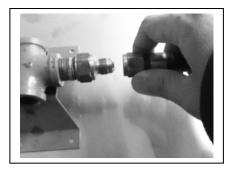
2-7) Install the factory supplied Natural Gas regulator directly and use pipe sealant approved for natural gas connection (shown below). Warning: The Natural Gas Regulator is set at 4" of Water Column.
