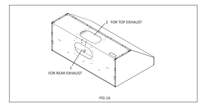
CAUTION: When knock outs are removed the edges will be sharp!!! Sharp edges should be filed or covered with metal tape.
