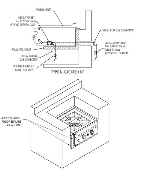
\* When Installing, use front right knockout to keep power cord cool. If using LP gas cylinder and insulating jacket (DHIJ), use stainless flexible hose to connect LP gas cylinder to grill Regulator.
